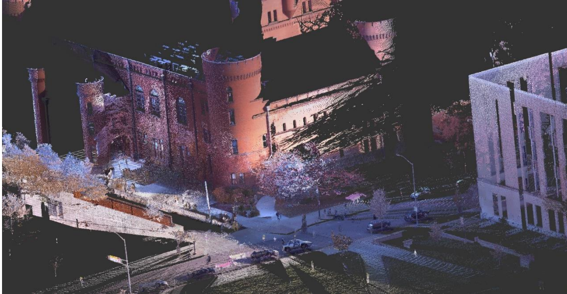
Point cloud data obtained by laser scanning using the Trimble x7 then imported into Autodesk Recap. The building scanned is the Red Gym, located in Madison, Wisconsin. (Corbett & Her, 2023).
