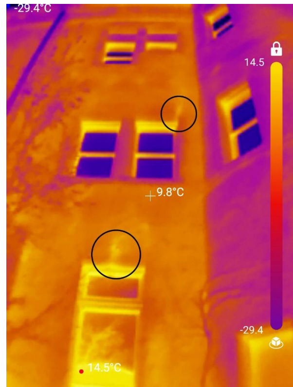
Thermographic images with hidden cracks.
