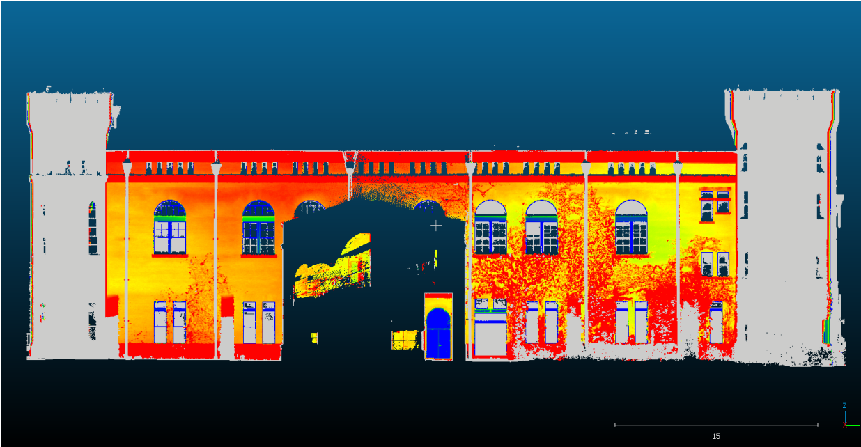
Using scalar fields in Cloud Compare to assess west wall deformation.
